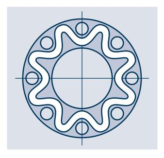
If there is considerable unevenness or damage to the sealing surface, thicker strips should be used. Due to the greater width that thicker strips have, a corresponding increase in the bolt load is required.
