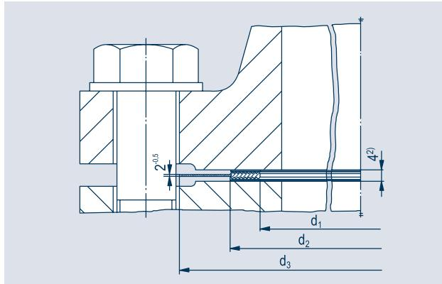
Works standard 145 = DIN EN 1514-6 for DIN flanges
