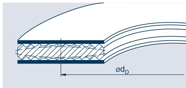
With gaseous media or large differences in temperature between the internal and external diameters, Profile B25A with loose sheet metal central edge should be used.
