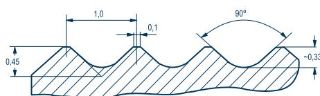
This profiling should be used with gaskets for flange connections with male or female faces or tongue and groove flanges. The minimum requirements are set out in our works standard WN 123.
