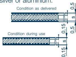
We recommend PTFE or graphite as layers for pipelines, apparatus parts or valves made from austenitic materials. The layers should be either attached without glue or a low-chloride adhesive should be used.
