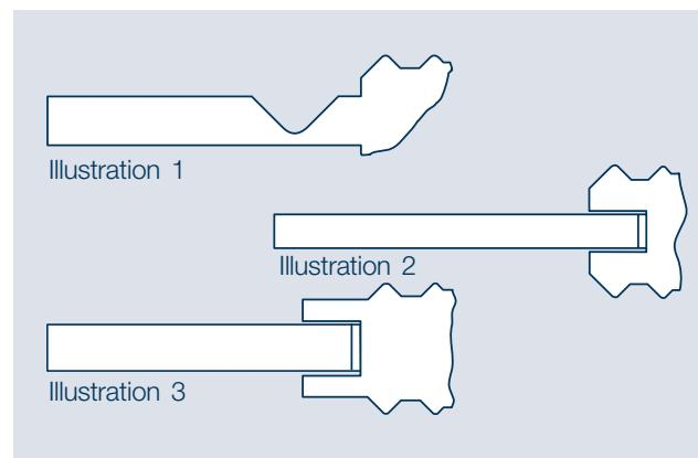
Grooved gaskets are available that conform to works standards WN 100, WN 101, WN 136, WN145 (DIN EN 1514-6), WN 146 and WN 147. Works standards 100 and 101 only contain a sealing width for all nominal pressure levels.
