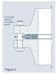
Old and new plants constantly place greater demands on safety and reliability. This applies at certain sizes to bolted flange connections on apparatuses, valves and pipelines. For many years, sealing systems with intermediate exhausting or certain areas of the chemical industry. The simplest example of this consists of two O-rings concentrically arranged in grooves.
