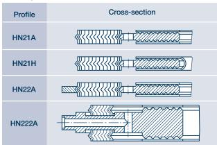
The standard material for the metal carrier of the inner gasket and for the metal strip of the spiral gasket is 1.4541 or 1.4571 steel. Other materials available on request. See also the section "Materials commonly used".
